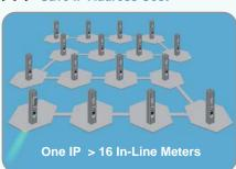
InfraPower In-Line Meter is designed to support daisy chain connections. It allows up to 16 In-Line Meters to be cascaded via Cat6 cables - All the PDUs with In-Line Meters are remotely accessed via a single network IP.
