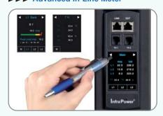
InfraPower In-Line meter provides the cascade ports for network connection. Two sensor ports are integrated for temperature & humidity monitoring. The 2.8" touchscreen LCD offers a real time local PDU monitoring.
