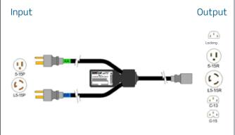
The **Zonit Z-ATS MICRO** is easily configured for your specific use case by changing the cord length, cord color and plug type (including locking or non-locking configurations).
